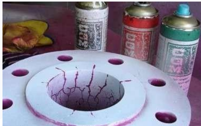
Dye Penetrant Testing
